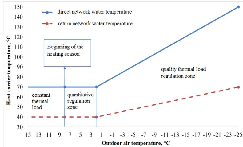
Figure 4: Temperature scheme of district heating 150/70 °C
