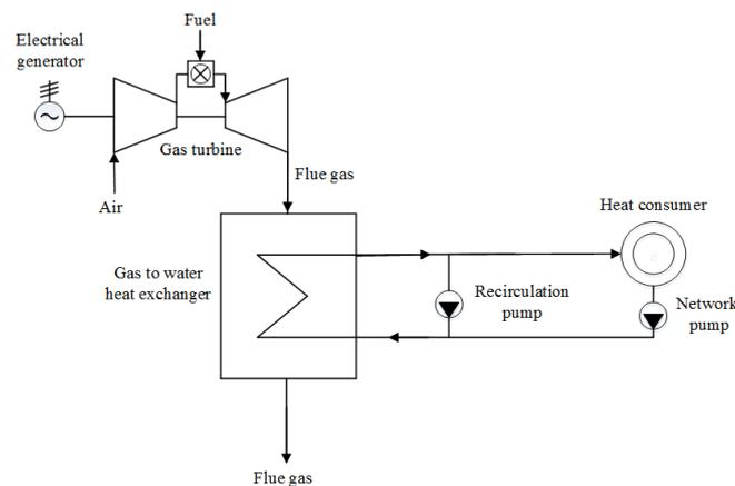
Figure 2: Thermal scheme of GT CHP with recirculation line of GWHE
