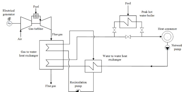
Figure 6: The second thermal scheme of heating GT CHP
