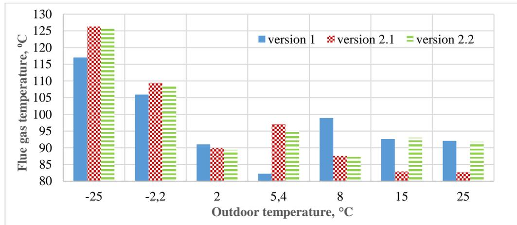
Figure 9: Dependence of the flue gas temperature on the outdoor temperature
