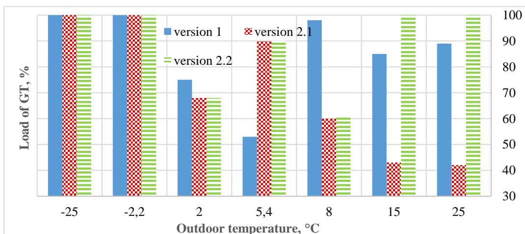
Figure 8: Dependence of the total load of the gas turbine on the outside temperature
