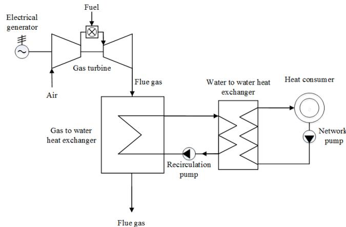
Figure 3: Thermal scheme of GT CHP with intermediate WWHE
