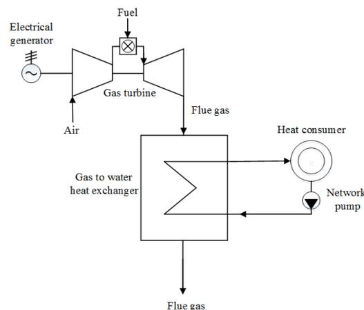
Figure 1: Elementary thermal scheme of GT CHP
