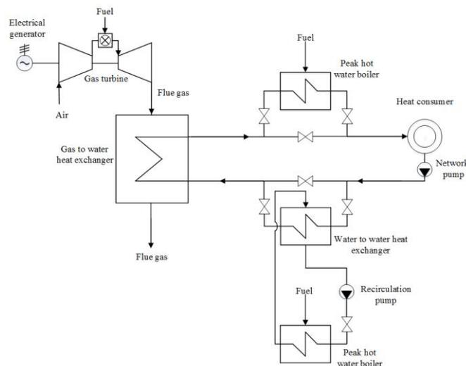
Figure 5: The first thermal scheme of heating GT CHP
