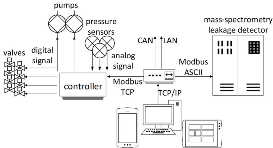
FIGURE 2 The control circuit of the computer based automated remote leakage detection system.
