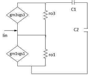
Figure 4: Small signal model for input section
