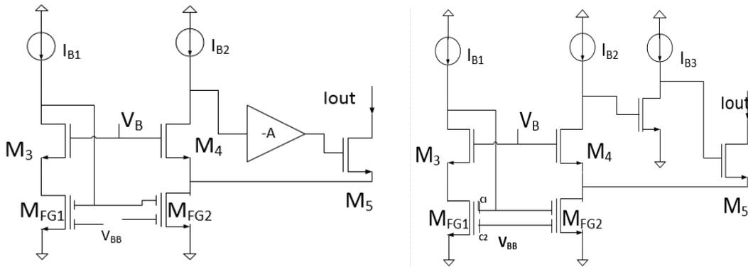
Figure 2: Proposed low voltage current mirror. Figure 3: Proposed low voltage current mirror with inverting amplifier implementation.
