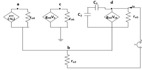
Figure 5: Small signal model of output section
