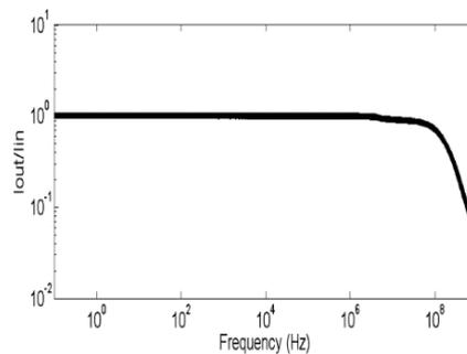
Figure 8: Frequency response of proposed current mirror
