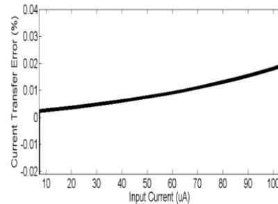
Figure 7: Error in current transfer
