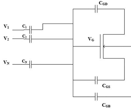
Figure 1: Symbol of floating gate MOSFET.
