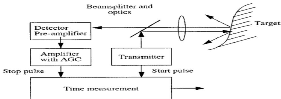
Fig. (1) Block diagram of TOF laser range finder
