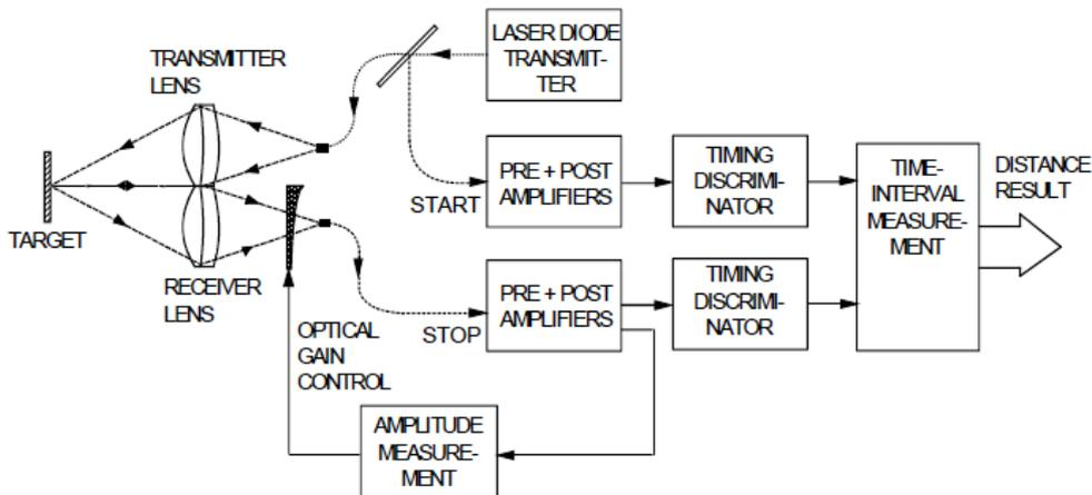
Fig. (2) The structure of a two – channel TOF laser range finder
