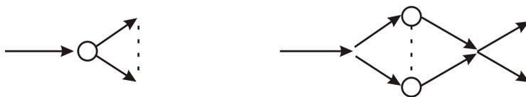
Fig. 3. Transformation of system with hyperexponential service times distribution into network with exponential times distributions.
